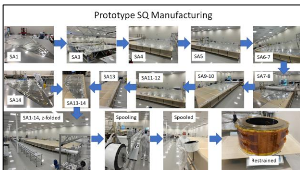
Figure 9. Collage of prototype SQ manufacturing and packaging
